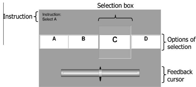
Fig. 2. Graphical user interface for the BCI test.
